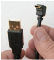
A USB A to a Down Angle Mini-B cable (not included) is needed in order to connect the camera and set the camera adjustments using the USB application.
